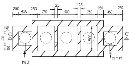
DETAIL OF SEPTIC TANK FOR 30 USERS SCALE - 1:50
